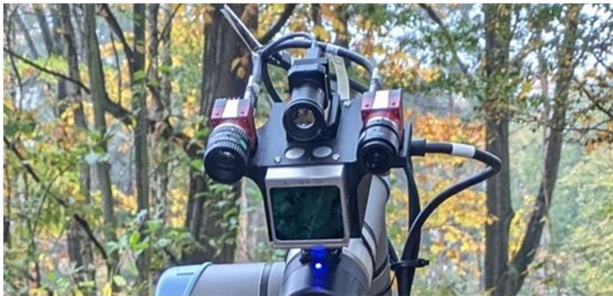
Figure 2. Example of multi-spectral (RGB, SWIR, LWIR) camera and LiDAR payload for object detection
